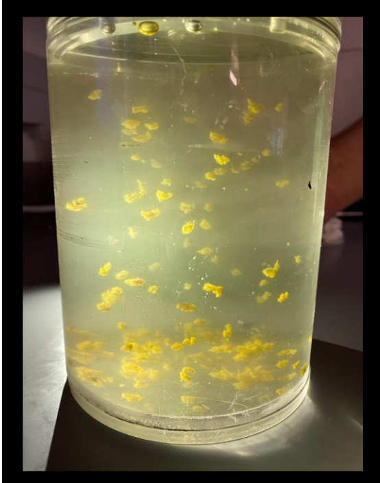
Roller tank (1.5 L) with marine snow
