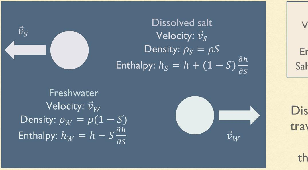
Mixture: Seawater Velocity:  $\vec{v} = S\vec{v}_S + (1-S)\vec{v}_W$ Density:  $\rho$ Enthalpy:  $h = S h_S + (1-S)h_W$ Salt Flux:  $\vec{J}_S = S(1-S)(\vec{v}_S - \vec{v}_W)$
