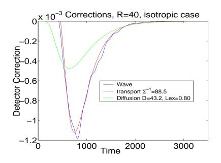
Wavelength  $\lambda=1$ , mean free path  $\approx 40$ , isotropic cross section.
