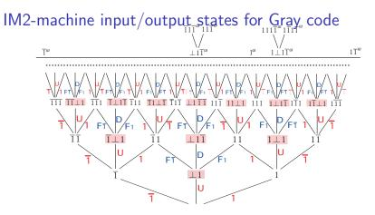
Two states G (normal state) and H (auxiliary state, red in picture).
